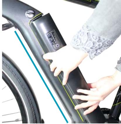
2. Place the battery catches into the dents provided.
