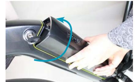
4. Turn the battery key clockwise. Now the battery is locked.
