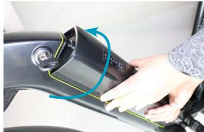
4. Turn the battery key clockwise. Now the battery is locked.
