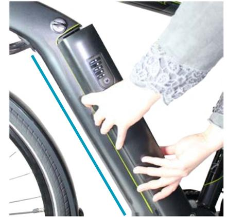
2. Place the battery catches into the dents provided.
