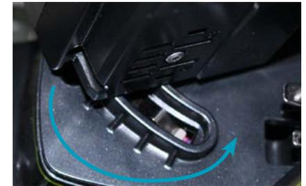
3. Roll the battery into the docking station until it clicks into place.
