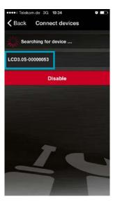
6. Select the S-Pedelec you want to connect to your smartphone. The number of your S-Pedelec is on the back of the display. This is an 8-digit serial number. Use the last digits of the number.
