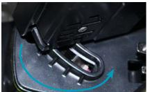
Roll the battery into the docking station until it clicks into place.
