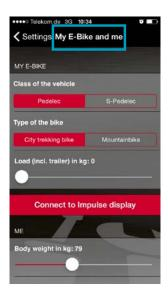
**5.** Select "Connect to Impulse display". The App starts to look for the S-Pedelec. After a short time, all Bluetooth-capable S-Pedelecs are displayed in the form of a number combination.
