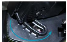
3. Roll the battery into the docking station until it clicks into place.
