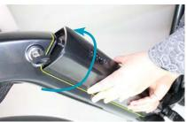
4. Turn the battery key clockwise. Now the battery is locked.
