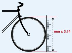
**2.** Push your cycle by one full revolution and measure how far it travels (in mm).
