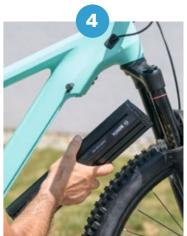
Push the top of the battery to detach it the from the restraint support – the battery then falls into your hand.
