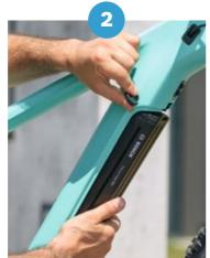
The battery is unlocked using a key and then falls into the restraint support
